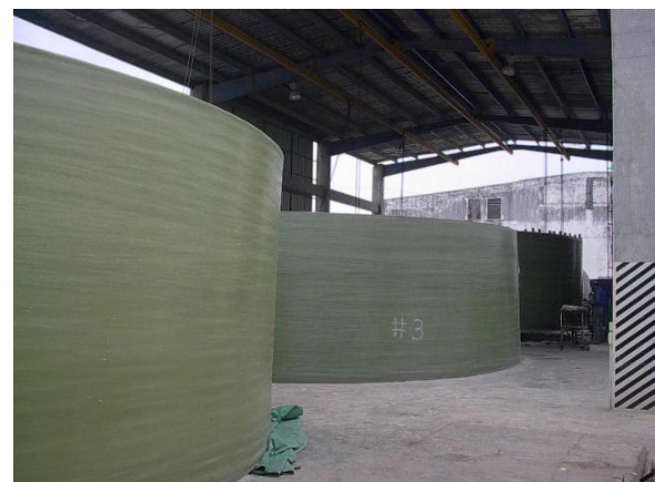
Shop fabrication of floor and wall sections of 350,000 gallon FRP tank
