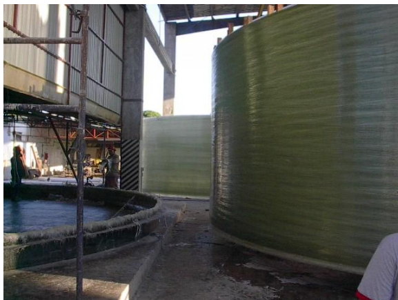
Shop fabrication of floor and wall sections of 350,000 gallon FRP tank
